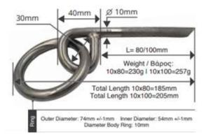
They are tested according to EN 959:2018 designed for use as rock anchors. Rock anchors are defined as anchor devices insert in a rock hole, held in place by epoxy glue and with an attachment point for a connector. The anchor device is tested according to UIAA 123\_3 - rock anchors.
