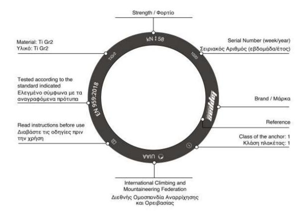
When used for CRONUS, the marking of RHEA is not applicable, the user must only refer to CRONUS marking on the ring. Marking of RHEA device is applicable when used alone.
