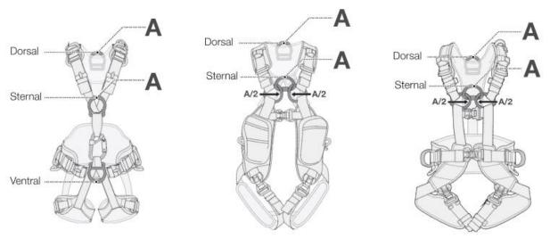
Instruction: A Full body harness is the only acceptable body holding device that can be used in a fall arrest system.
