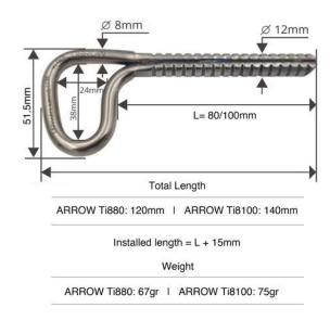
They are tested according to EN 959:2018 designed for use as rock anchors. Rock anchors are defined as anchor devices insert in a rock hole, held in place by epoxy glue and with an attachment point for a connector. The anchor device is tested according to UIAA 123\_3 - rock anchors.
