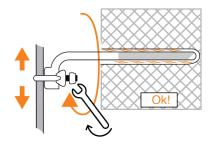
Clamp Torque: 40Nm Safety Line Diameter: 12mm
